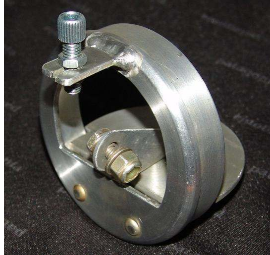
Modified jar lid to balance the Turbo System (Airbox)
