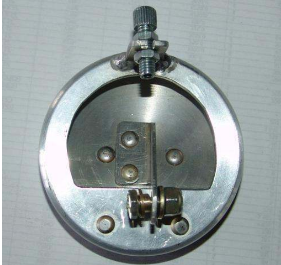
Modified jar lid to balance the Turbo System (Airbox)
